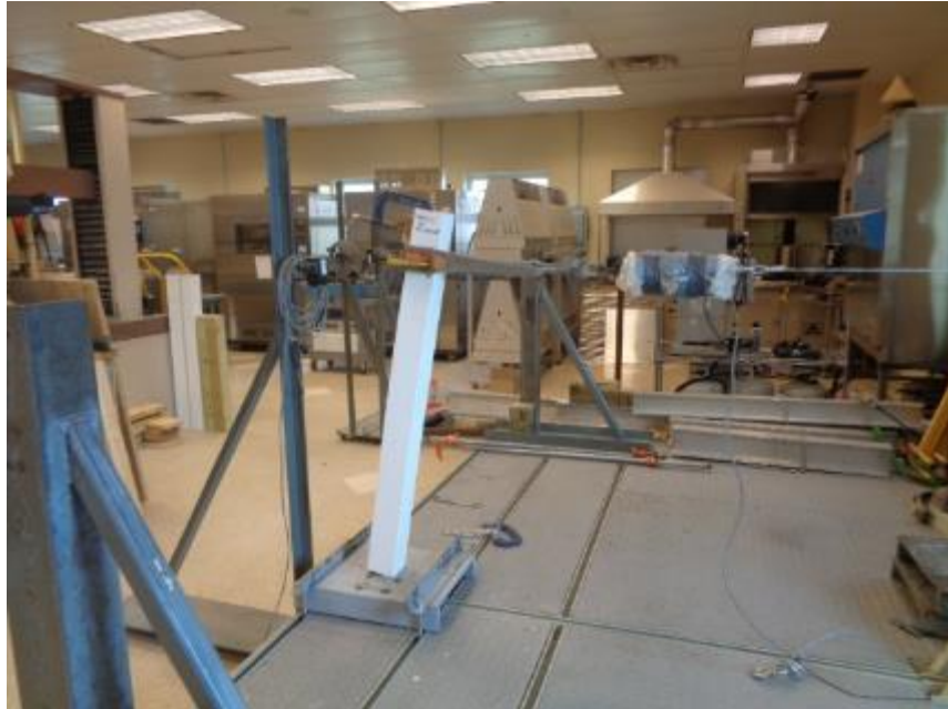
Photo No. 3 Concentrated Load Test at Top of Post Mount Simulated Concrete
