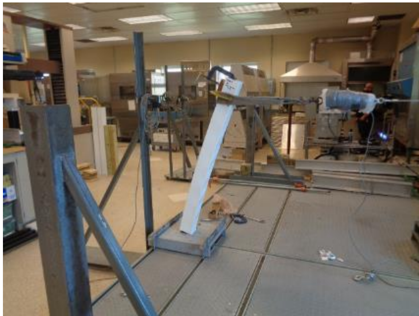
Photo No. 4 Concentrated Load Test at Top of Post Mount Simulated Concrete Bolted Through Bottom Spacer
