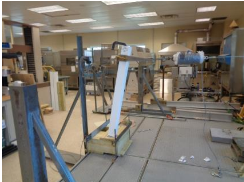
Photo No. 2 Concentrated Load Test at Top of Post Mount Mock Wood Deck
