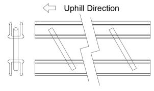
c. Place the Top and Bottom Common Rail together and pass two balusters through the routed holes to ensure the hole patterns are properly aligned. Make a single cut across each end of the Common Rails, at the locations/angles. Note: do not cut the Rail Top Cap until section is assembled and secured at all 4 mounting points.
