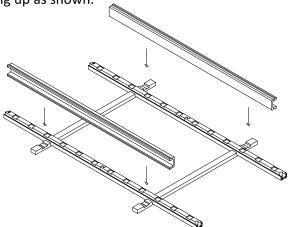
3. Lay the common rail sections on their sides in the outer routed pockets as shown.
