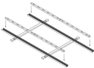
2. Locate the Baluster spacing jigs and press them together using the connectors on the end. They should fit together snugly. Then place them within the gap of the aluminum reinforcements with the routed pockets facing up as shown.
