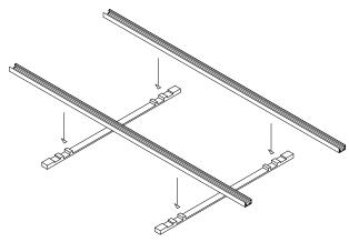
1. Using saw horses or other flat work surface, lay out the routed guide boards in parallel. Take the aluminum reinforcement lengths and lay them in the appropriate channels as shown. Note that channels are included for both 36" and 42" rail height.
