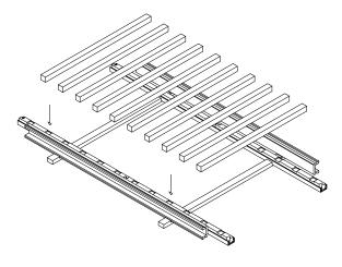
4. Determine the appropriate centering for the common rail sections, secure them in these positions, and begin laying balusters in the baluster guides as shown.
