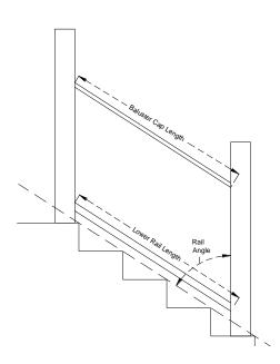
Note: IBC code requires that finished stair rail heights be a minimum of 34" plumb off the nose of the tread. The standard RS35 36" rail kit's balusters will typically meet these requirements provided the rail is being installed with the bottom rail elevated above the stair treads. In the event that the railing is being installed directly at or slightly above the stair tread nose, INTEX recommends using the RS35 Stair/Rake Rail kit, which will meet the minimum height requirement any scenario.
