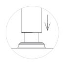
One post cover is predrilled for the Door Hinges. Ensure that this cover is positioned on the correct side of the post that will support the hinge side of the door.
